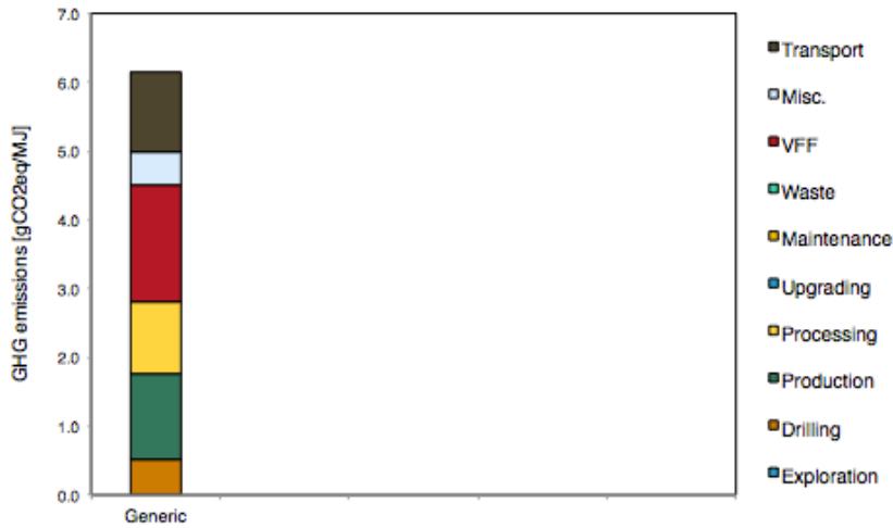
Figure 2.5: Graphical results for a 'Generic' crude oil. 'User Inputs & Results' Figure 1.1.
