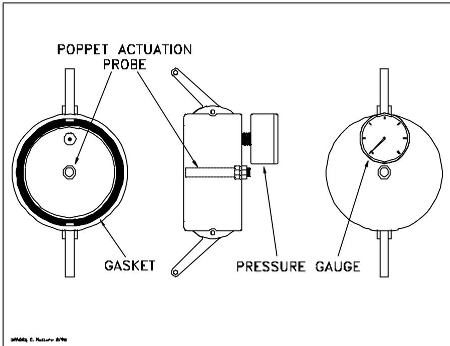
**Figure 3 - Vent Pipe and Vapor Return Meter Arrangement**
