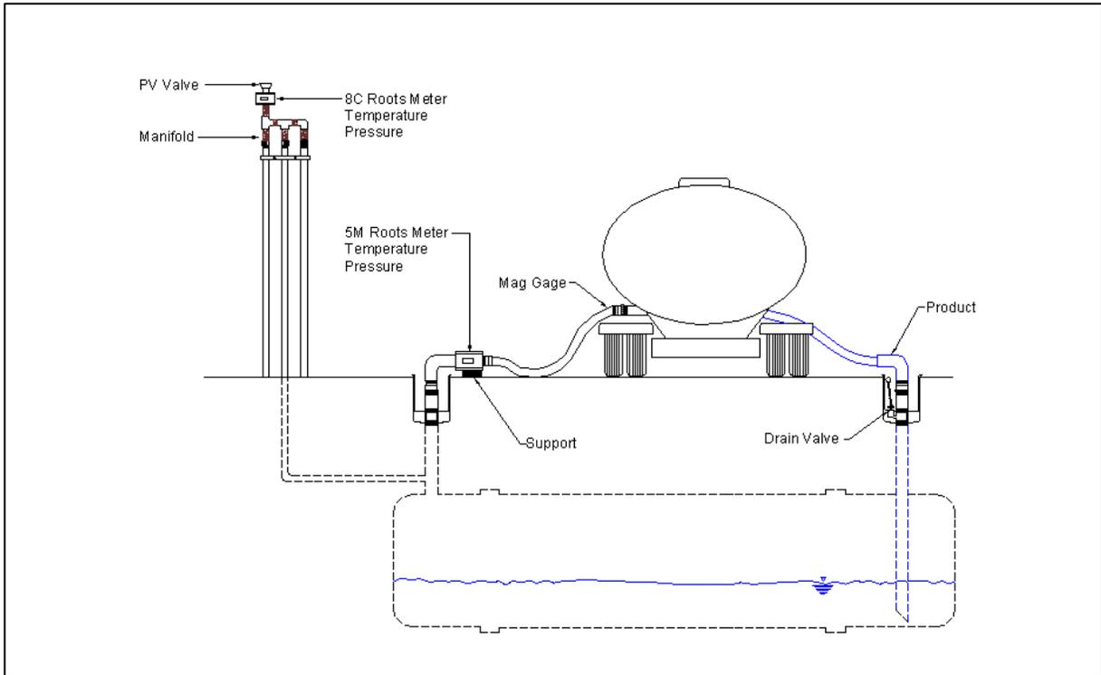
**Figure 4 - Example of A Steel Vent Pipe Manifold**
