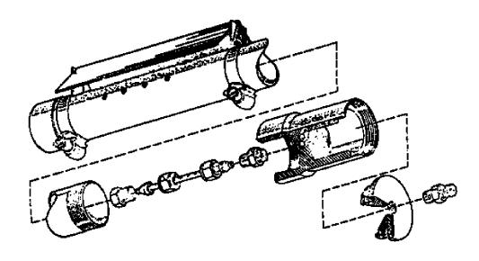
Figure 16-1. Probe Used for Sample Gas Containing High Particulate Loadings.
