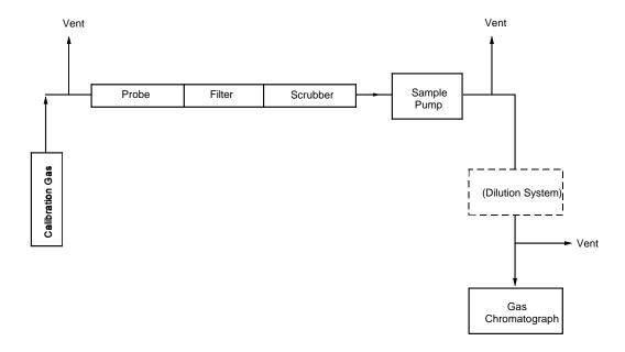
Figure 16-2. Determination of Sample Line Loss.
