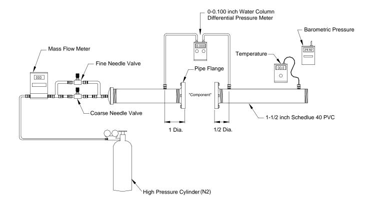
Notes: Three tube configurations are required to measure different components. Each configuration requires a uniquely designed orifice plate, flange, couplings, and male & female interfacing adapters.
