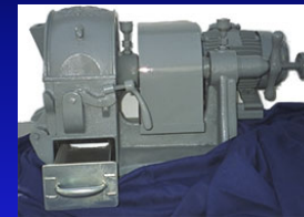
Braun Mill (plate grinder)
