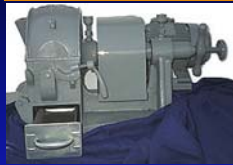
Plate Grinder (Braun Mill)
