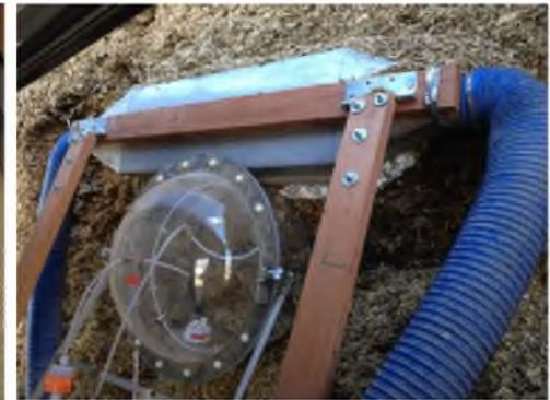
Wind tunnels and flux chambers for emissions measurements
