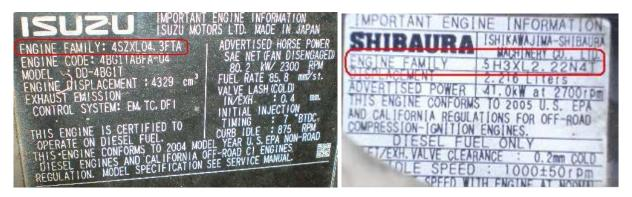
If the engine label is missing or cannot be located, contact the engine manufacturer for the location of the label or for a replacement label. The engine manufacturer may require the engine serial number in order to replace the label. The engine manufacturer can advise you as to where the engine serial number is stamped on the engine block. ARB staff will assume that an engine is a non-certified engine if it is without a label or EFN.
