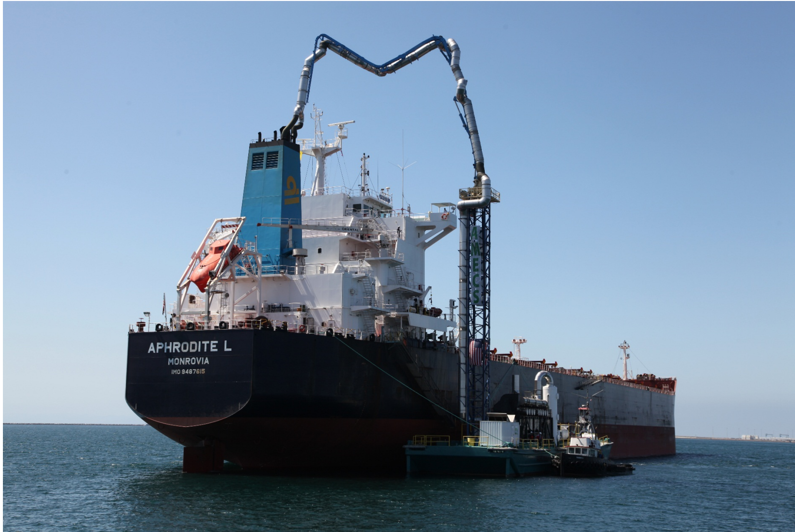
AMECS Barge System At-Ancor Direct-Connect Stack Exhaust Capture System
