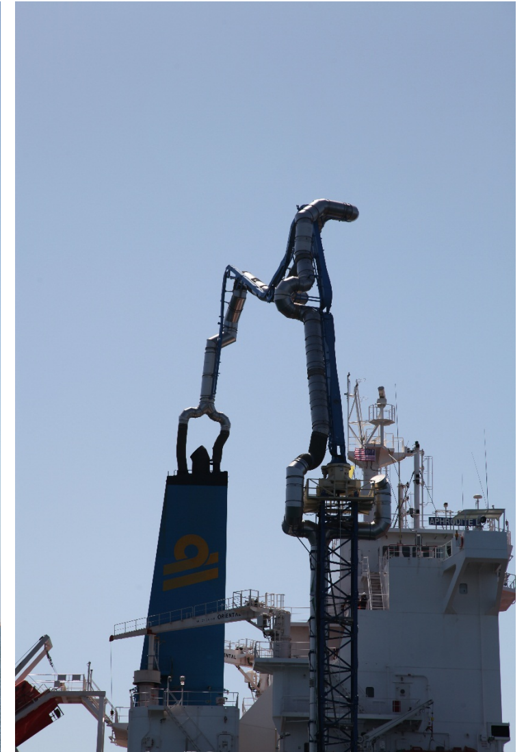
AMECS Barge System At-Ancor Direct-Connect Stack Exhaust Capture System
