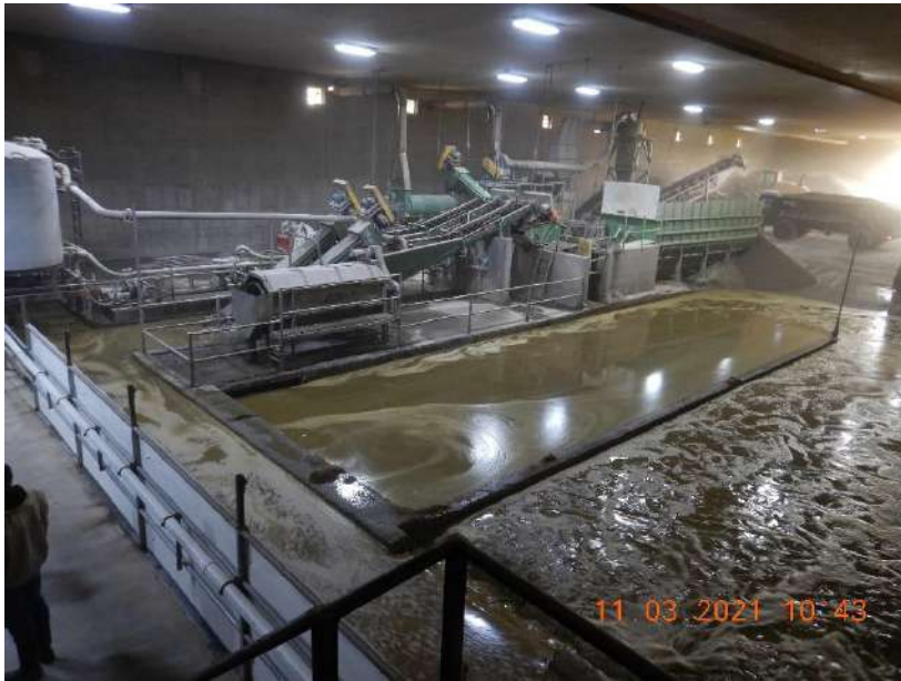
Photo 47. The sand separation building at Site 2. Sand bedding that enters the manure transfer system in the freestall barn at Site 2 is removed from the manure, cleaned, and stored in this location until it is reused for bedding.
