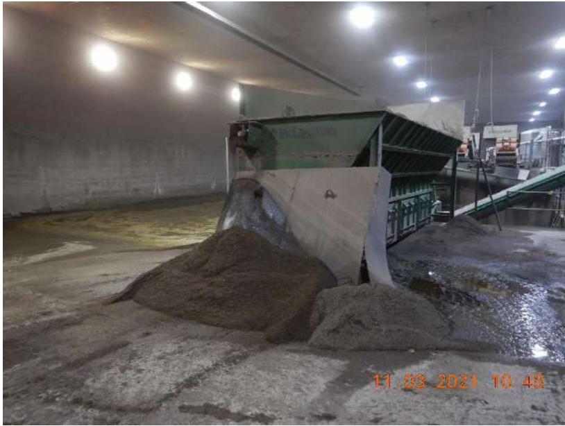
Photo 59. The sand separation building at Site 2. Sand bedding that enters the manure transfer system in the freestall barn at Site 2 is removed from the manure, cleaned, and stored in this location until it is reused for bedding.
