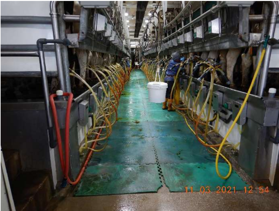
Photo 83. The milking parlor at Site 2. All process wastewater generated is captured and comingled in the manure transfer system.
