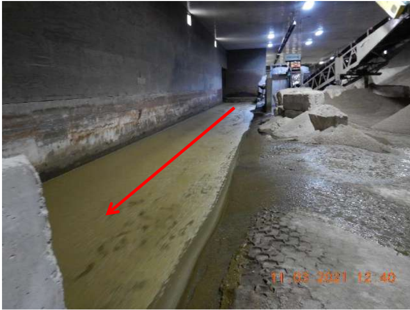
Photo 68. The flow path of manure through the sand separation building at Site 1, represented by the red arrows.
