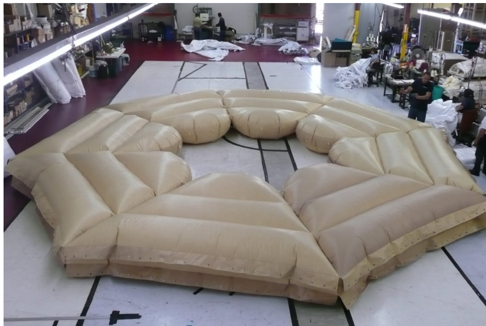
Figure 5. Octagonal Capture Bonnet's Pneumatic Interface Collar
