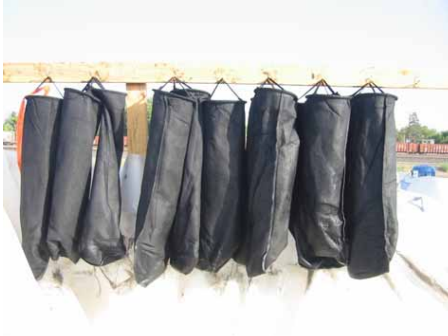
Figure 25. Some Solid Waste Filters Used During the Demonstrating Testing
