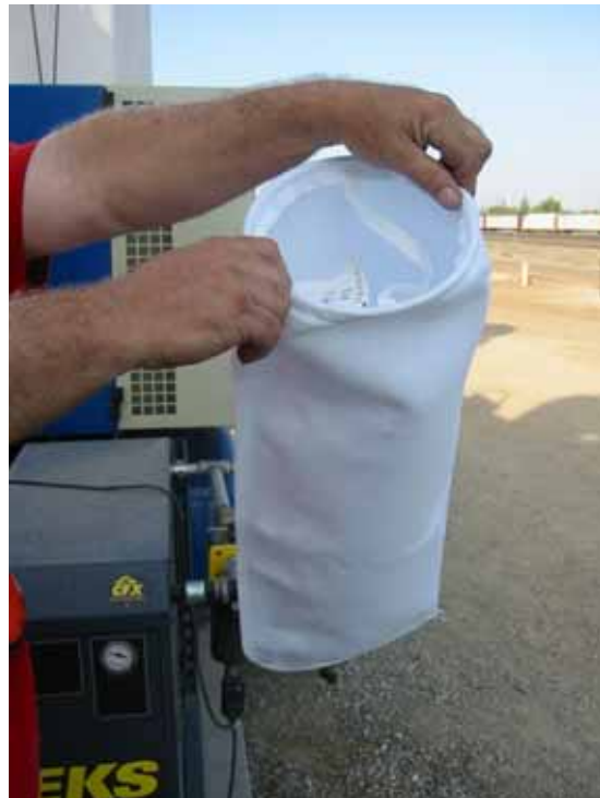
Figure 26. Clean Solid Waste Filter
