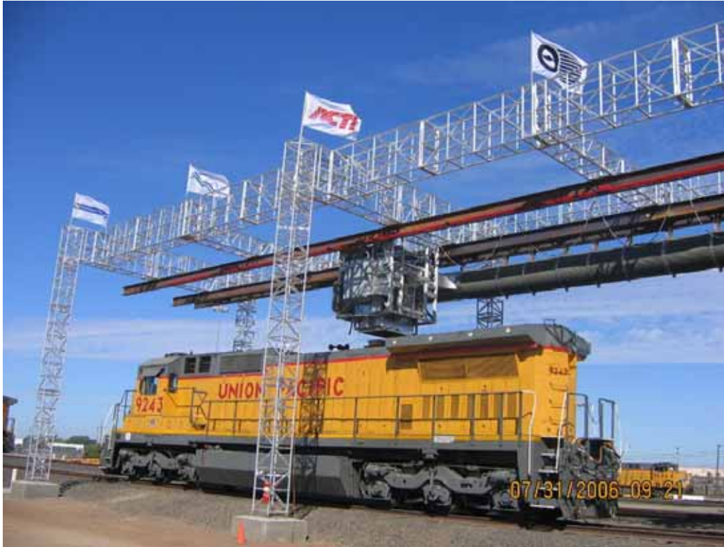
Figure 3. Locomotive under the Exhaust Capture Bonnet
