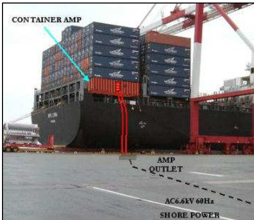
Figure IV-15: Shore Power Connection Using a Container Box
