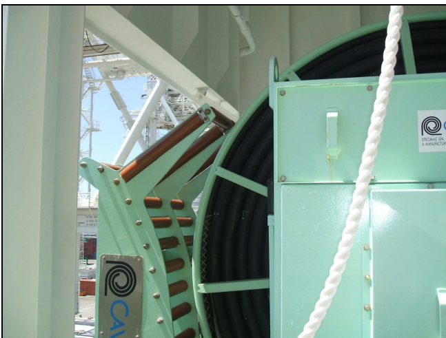
Figure IV-12: Cable Reel Onboard the Ever Steady
