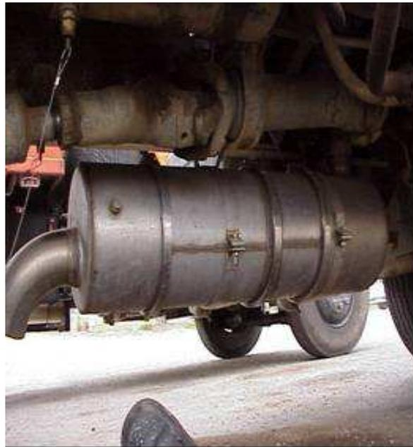
**Figure VII-6: Horizontal DPF Installation for Vertical Exhaust**
