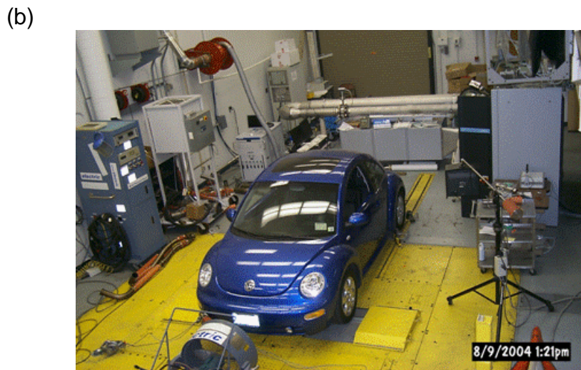
Figure 26. (a) Side view of ARB LDV emission laboratory setup shown the chassis dynamometer, the CVS dilution tunnel and the PM and gaseous emissions sampling trains. (b) Picture of test cell.
