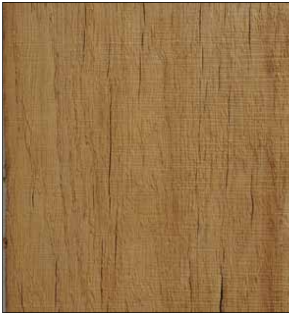
Figure 13-8. Surface checking on white oak 5/4 lumber.
