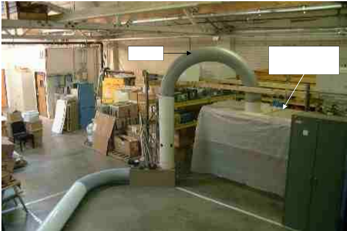
Figure V-1. Temporary 'Hood' for Capturing Hexavalent Chromium Emissions at Decorative Chromium Plating Facilities
