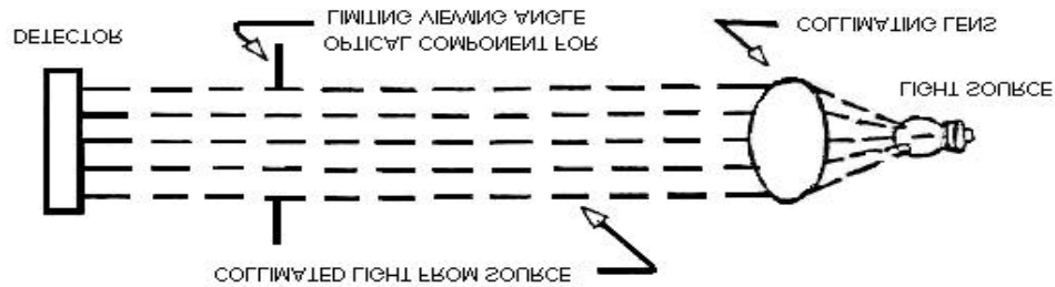
FIGURE 184-1 SMOKE METER OPTICAL SYSTEM (SCHEMATIC)
