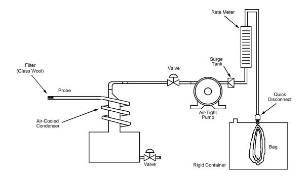
Figure 3-2. Integrated gas-sampling train.
