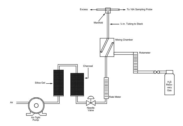
Figure 16A-3. Recovery Gas Dilution System.
