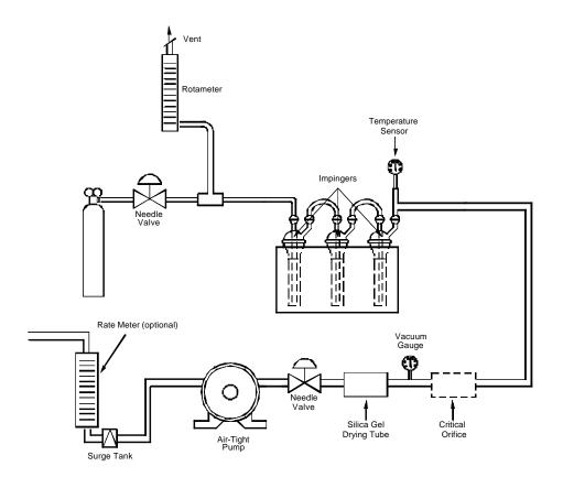
Figure 16A-4. Recovery Check Gas Sampling Train.
