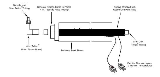
Figure 16A-2. Angled Sampling Probe.
