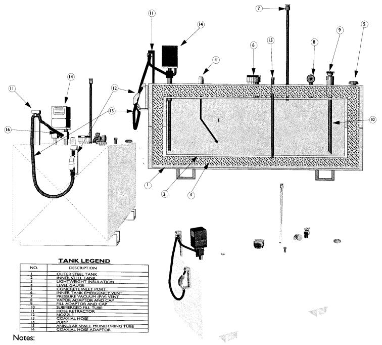
Tank construction shall include a minimum of 6 inches of concrete insulation between the interior holding tank and the exterior containment tank.
