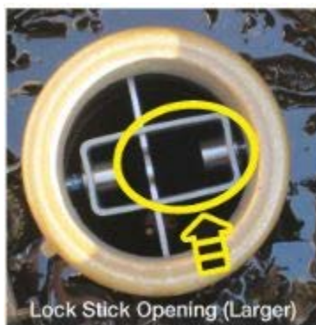
McGard Fuel Lock Installation Position 3
