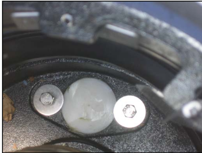
Figure 1-4 1DP-2100 Field Installed Drain Plug
